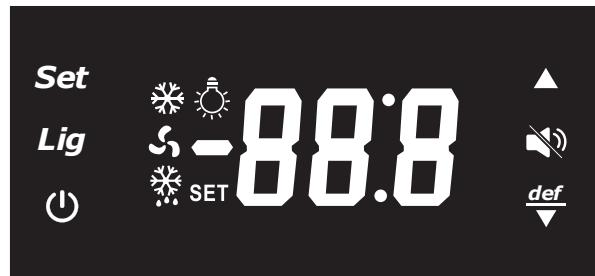
The controller has a range of 2 °C – 18 °C, with default setting of 5 °C. In order to adjust the set point please follow the steps below:
